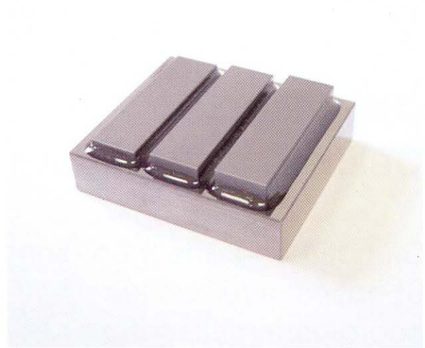
2-Stepped standard with diffuse reflecting measuring faces
