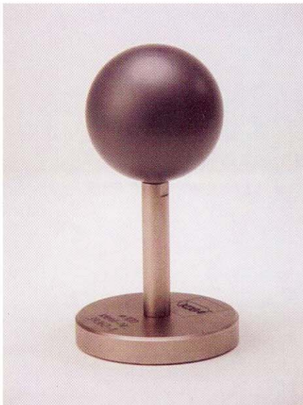
Sphere standard with diffuse reflecting surface
